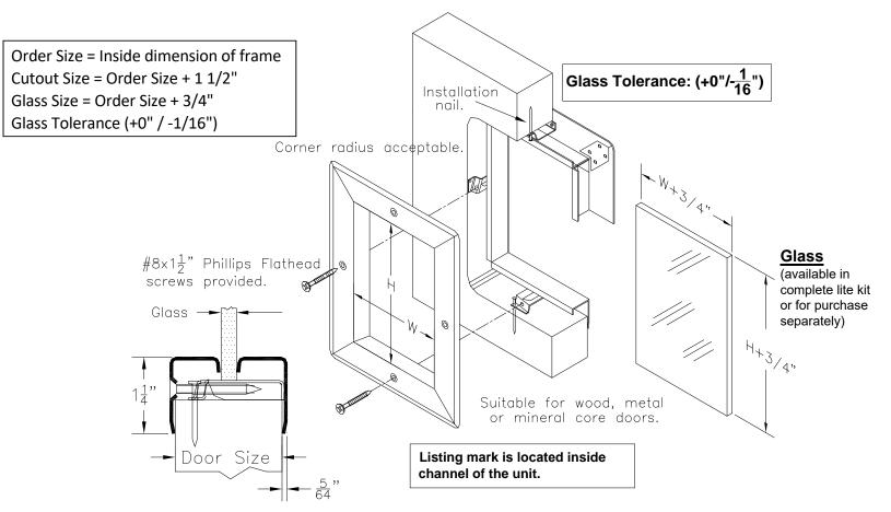
**NOTE ON GLAZING TAPE:** Some types of glass & some very large frames require glazing tape. Scan the QR Code (right) or visit www.allmetalstamping.com for a listing of approved glazing, fire ratings, or additional installation requirements such as tape or intumescent.
